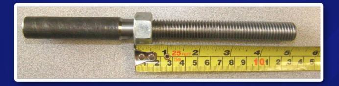
Thread length is measured to the end of a nut that is secured all the way up the threaded stud.
