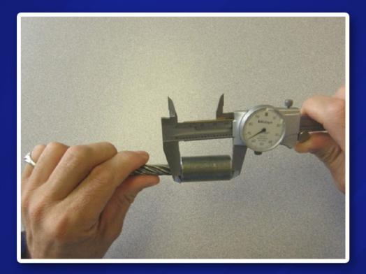
Measure the O.D. taking an average to account for flashing from the swaging process.
