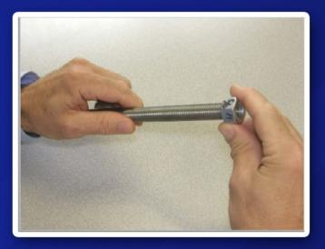
Measure thread outside diameter with caliper or with a nut that you know the size of.
